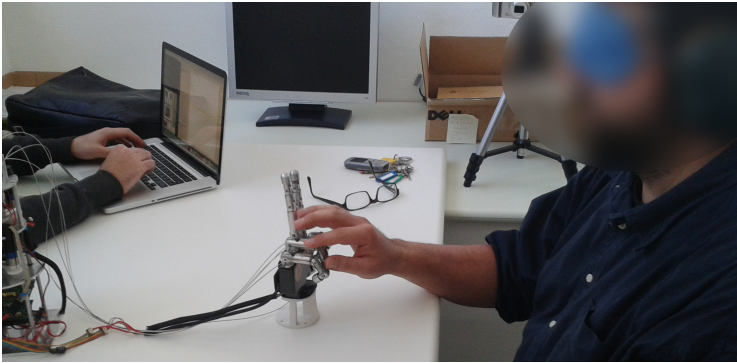
Fig. 9: Subject (blindfolded and with headphones) interacting with the robotic hand during the test session (V letter is performed in the picture).
