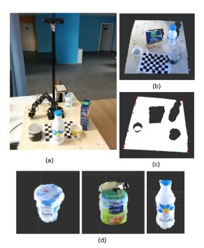
Fig. 2. Object detection pipeline. (a)The setup; (b) depth map of the table; (c) dominant plane; (d) segmented objects.
